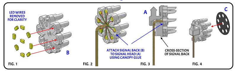
POSITION EACH LED / WIRE ASSEMBLY IN THEIR CORRESPONDING ROUNDEL OPENING IN THE SIGNAL HEAD (B) (FIG. 1). ATTACH IN PLACE USING CANOPY GLUE.
