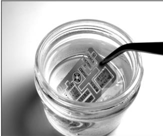
**The Entire Fret was dipped** into a solution of Black Oxide for Stainless Steel from EPI (Electrochemical Products Inc.)
