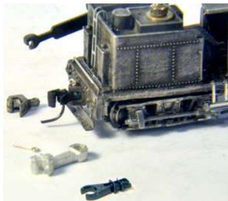
**Photo 13:** Coupler options: on the top in this photo is a Nelson Gray scale dummy coupler; next down, to the left, is the pewter coupler included in the kit which is MTL-compatible; attached to the locomotive is a shortened MTL 905 coupler; next down is a Pair Hands scale dummy knuckle coupler; below that (at the bottom of the photo) is an MTL “Civil War Era” link-and-pin coupler link, modified to fit the link-and-pin fitting on the Showcase locomotive.
