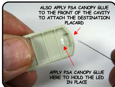
APPLY PSA CANOPY GLUE TO THE INTERIOR OF THE DESTINATION PLACARD CAVITY. ALSO APPLY PSA GLUE IN THE INDICATED AREA FOR PLACEMENT OF THE LED.
