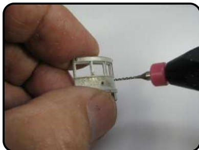
DRILL OUT THE HEADLIGHT OPENING USING A 1/32" DRILL BIT.
