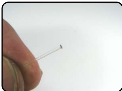
USING A SOLDERING IRON, CAREFULLY FLARE THE END OF THE INCLUDED FIBER OPTIC STRAND.
