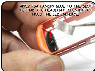
PLACE THE LED IN THE SLOT BEHIND THE HEADLIGHT OPENING AND APPLY THE METAL TAPE TO HOLD IT IN PALCE
