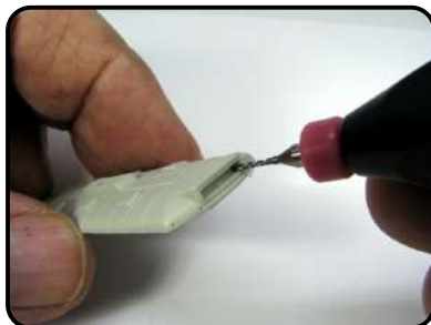
DRILL OUT THE DESTINATION PLACARD OPENING WITH A 1/32" DRILL. CLEAN UP OPENING WITH XACTO BLADE
