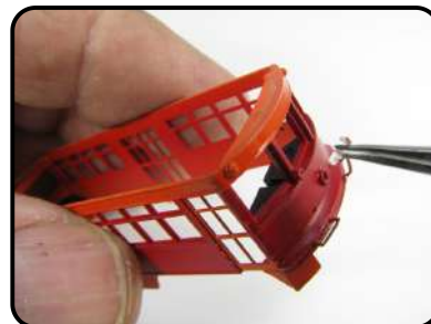
INSTALL THE FIBER OPTIC LENS INTO THE HEADLIGHT OPENING AND SECURE WITH PSA CANOPY GLUE.
