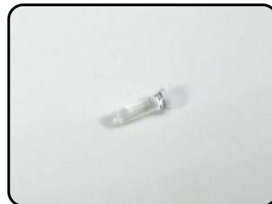
CUT THE FIBER OPTIC STRAND TO 1/16" TO 1/8" BEHIND THE LENS FLARE.
