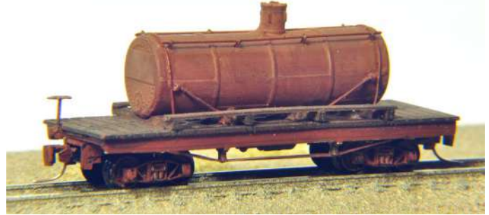
Photo 2: Completed tank car kit, heavily weathered. I added the tie-down rods which loop over each end of the tank, and the diagonal rods which prevent the tank from shifting fore-or-aft, which show in the historic photos of tank car No. 2.
