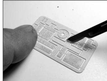
**Once the paint is COMPLETELY Dry** the paint on the raised detail was carefully scraped off the surface using a curved knife blade or 600 grit emery cloth (sand paper).
