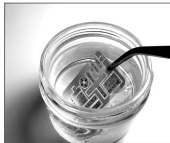
**The Entire Fret was dipped** into a solution of Black Oxide for Stainless Steel from EPI (Electrochemical Products Inc.)
