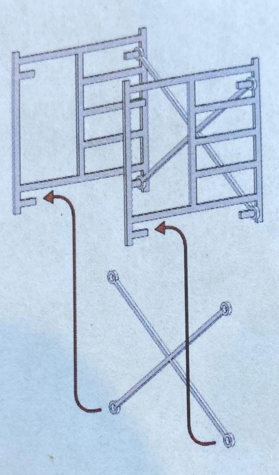
N Scale #523 and Z Scale #4018 Typical Assembly
