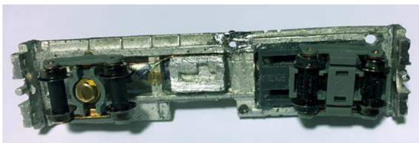
Photo 7: This bottom view shows the 00-90 screw which holds the boiler casting in place to finalize alignment prior to gluing it in place. Also visible are the holes for attaching the water tank and the cab.
