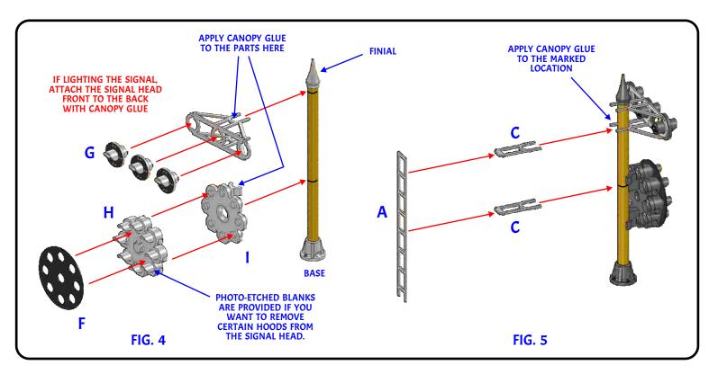
ATTACH YOUR CHOICE OF FINIALS TO THE TOP OF THE MAST TUBE AND THE BASE TO THE BOTTOM. GEL TYPE CA GLUE WORKS BEST FOR THE FINIAL AND THIN CA FOR THE BASE.
