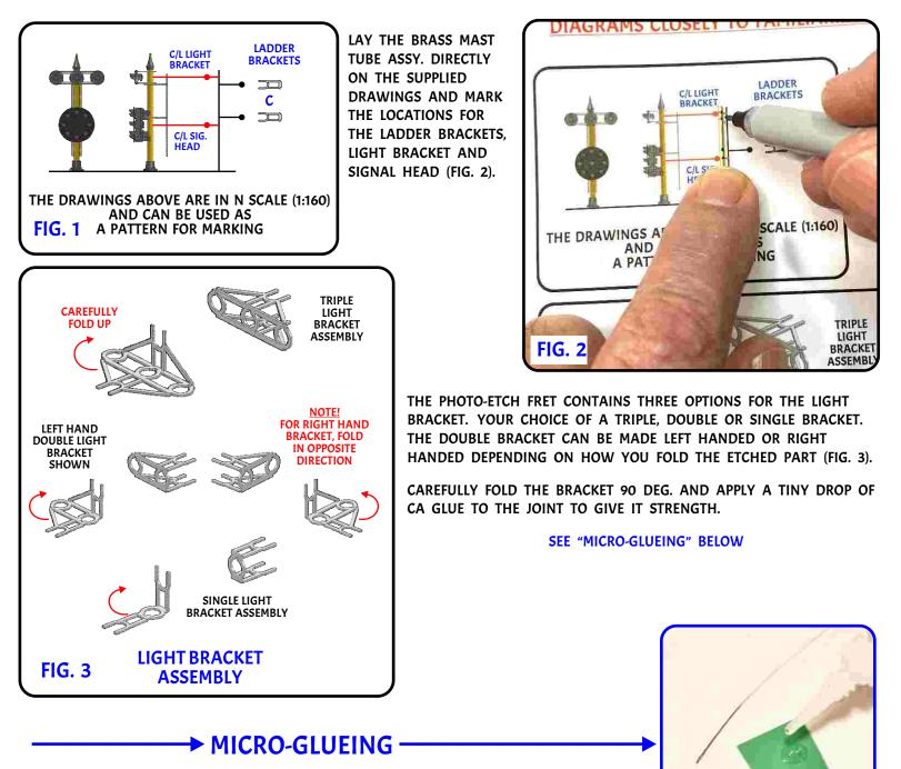
APPLY SEVERAL DROPS OF SUPER GLUE TO A PLASTIC SURFACE FOR A RESERVOIR AND USE A SHORT LENGTH OF FINE WIRE TO DIP OUT A TINY DROP OF GLUE (FIG. 8).
