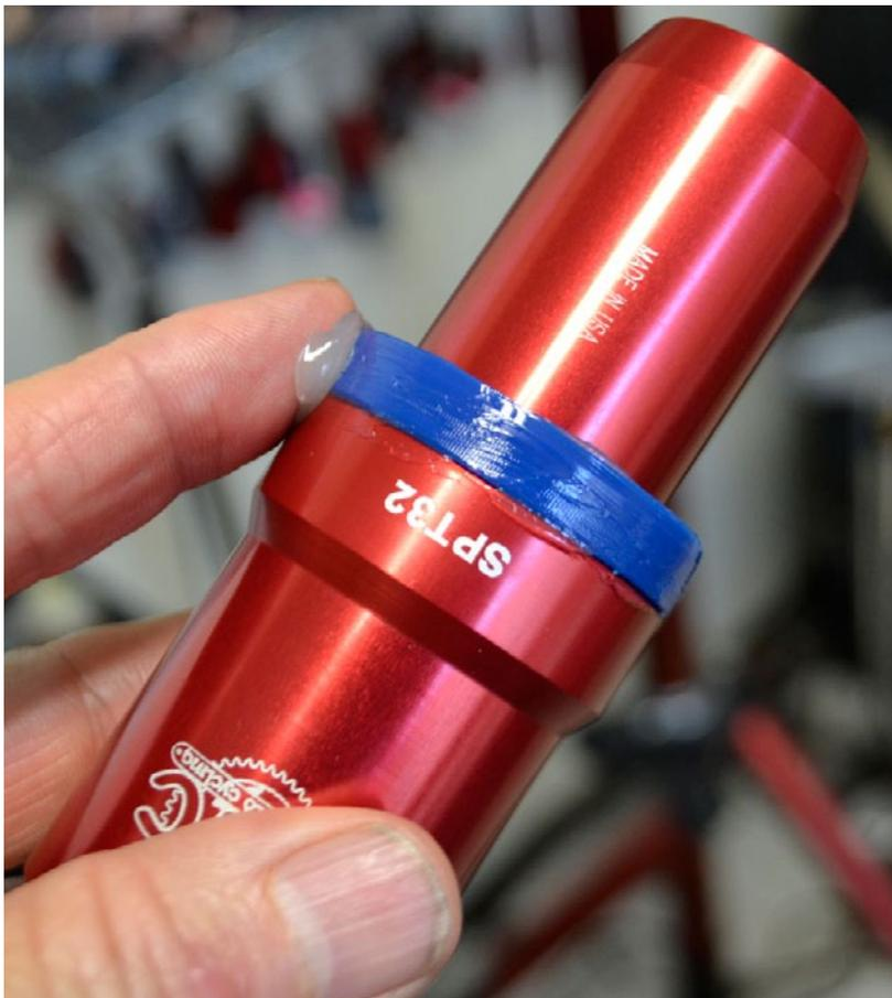
Grease the outer edge of the new wiper.
