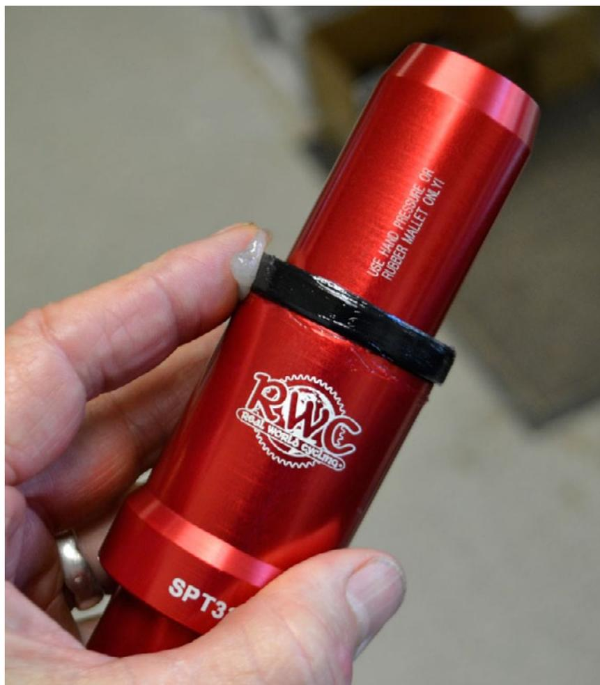
Start the pilot of the seal press tool into the upper bushing of the fork until the oil seal is resting inside the seal head.
