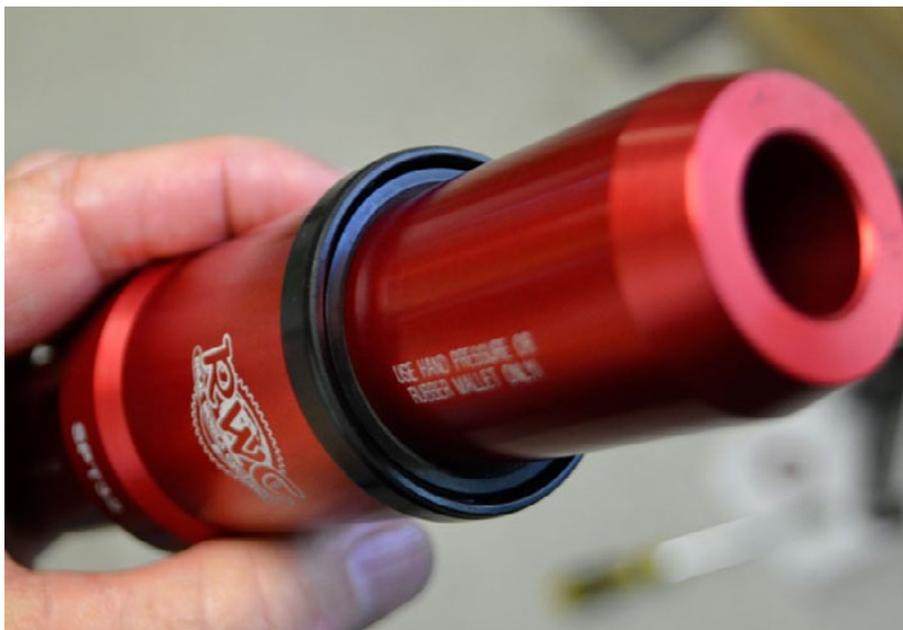
We highly recommend the use of our seal and wiper press tool. Place the new oil seal on the flangeless side of the press tool.
