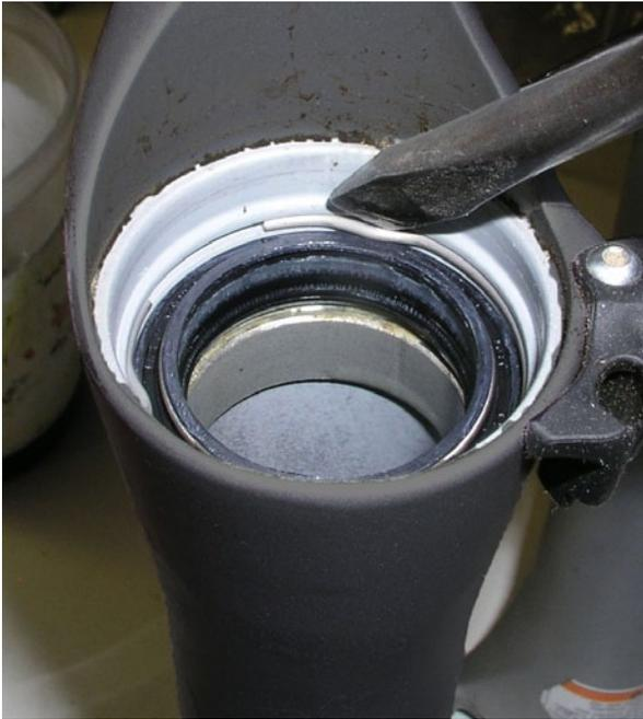
Replace the oil seal retaining clip into its groove in the seal head. Be sure that the clip fully expands into the groove *all the way around*.
