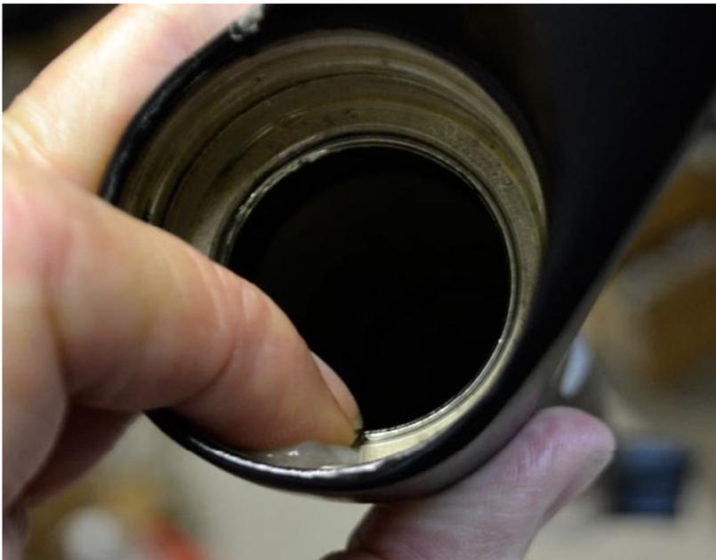
Use a suspension assembly grease such as Slickoleum or Rock 'n' Roll Super Slick grease to grease the inside of the seal head.
