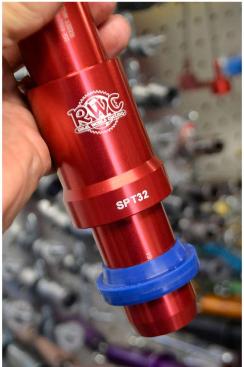
Slide the wiper up the press tool until the leading edge of the wiper is under the flange.
