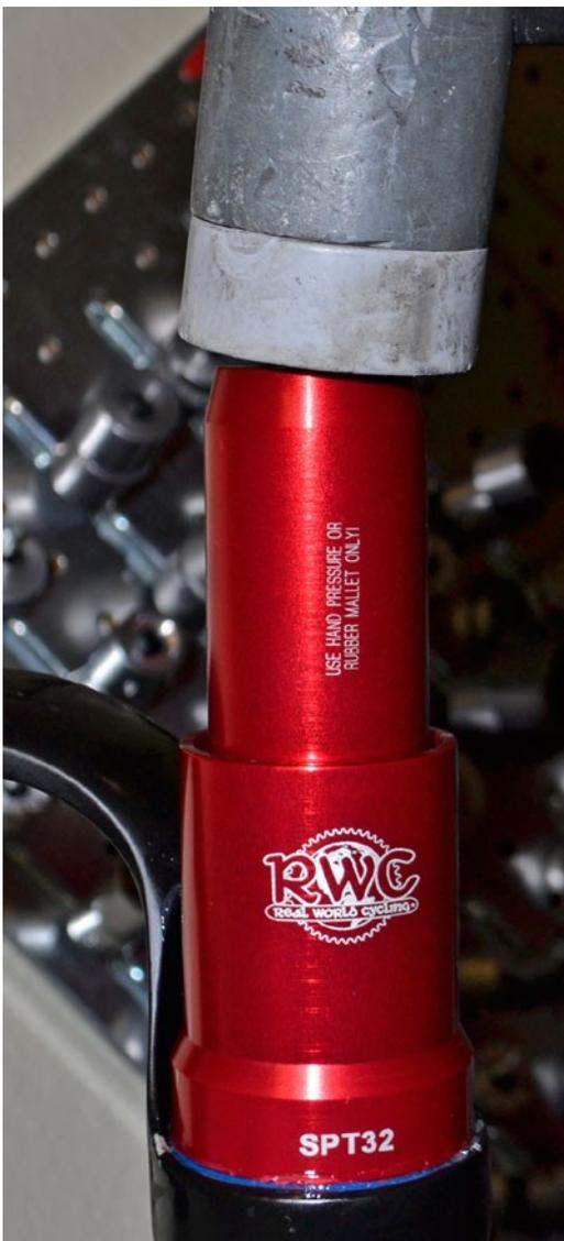
Rest the bottom of the fork legs against a padded, firm surface (a couple of folded up shop towels on top of a workbench will do).
