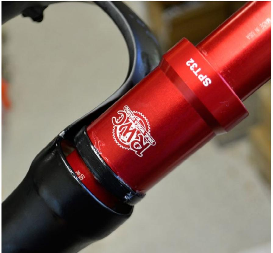
Rest the bottom of the fork legs against a padded, firm surface (a couple of folded up shop towels on top of a workbench will do).
