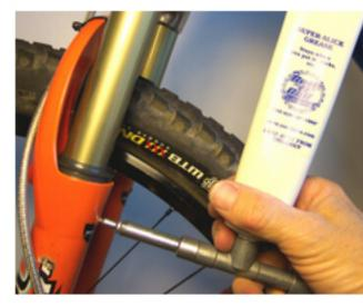
Add a few squirts of <u>"SUPER-SLICK GREASE"</u> into each Microlube port and cycle the fork a few times. Wipe any excess lube off of the stanchions, and you are ready to "break in" your new wipers.
