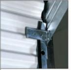
12-gauge, zinc-coated door stops are mounted to brackets for increased strength and ease of installation. 18-gauge, zinc-coated steel guides with polypropylene runners allow doors to glide easily.
