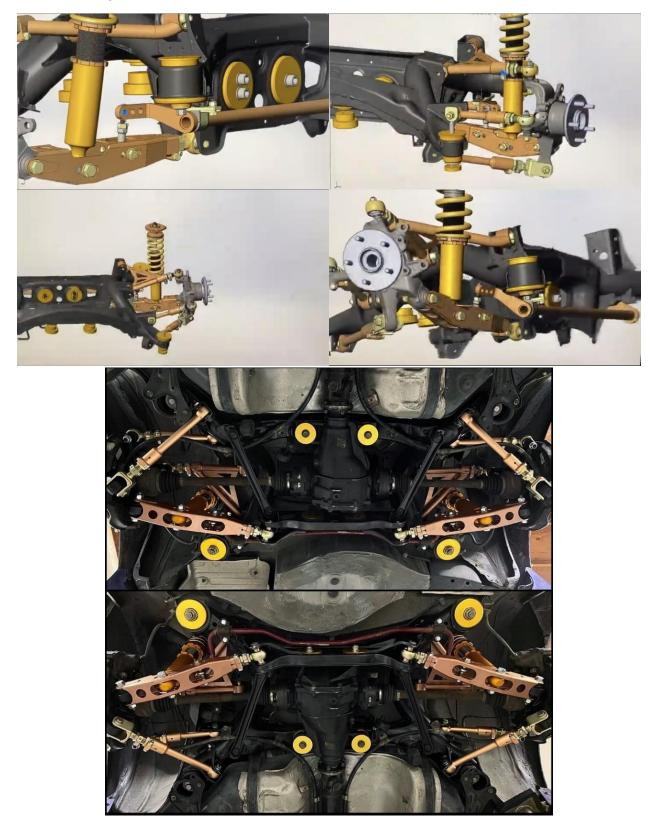
Clamping rod end receiver & Double Adjuster. Jam nuts (if used) lock against clamps. M22 nuts of lengths up to 55mm can cover rod end exposed thread.
