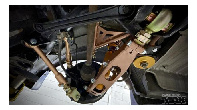
Clamping rod end receiver & Double Adjuster. Jam nuts (if used) lock against clamps. M22 nuts of lengths up to 55mm can cover rod end exposed thread.
