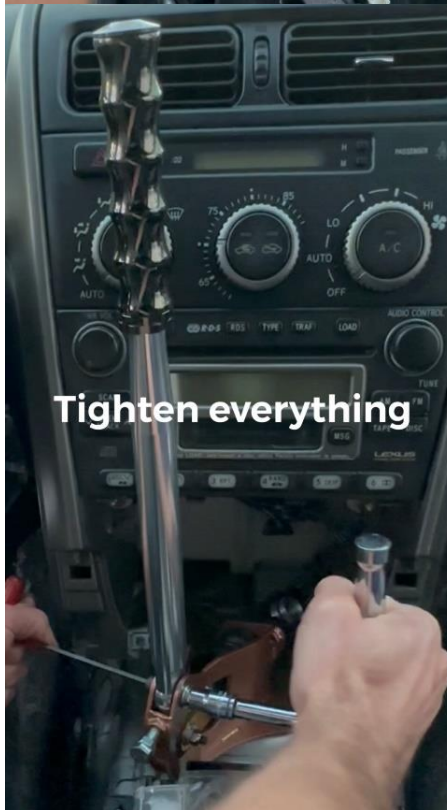
Set the handle angle With bump stop bolt.
