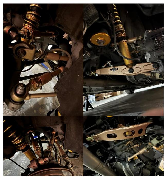
Clamping rod end receiver & Double Adjuster. Jam nuts (if used) lock against clamps. M22 nuts of lengths up to 55mm can cover rod end exposed thread.
