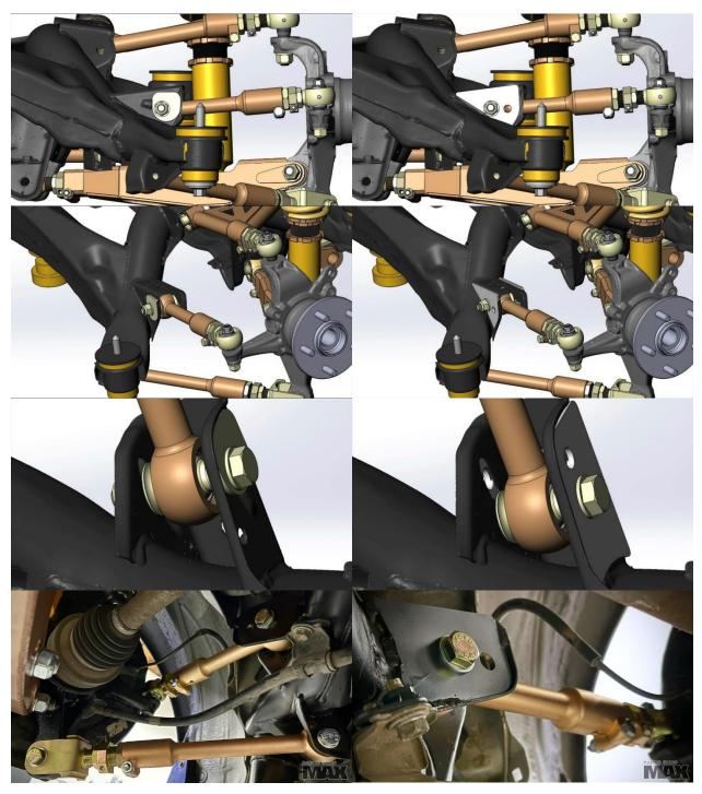
Install Example, compared to the weld on zero toe change plates.
